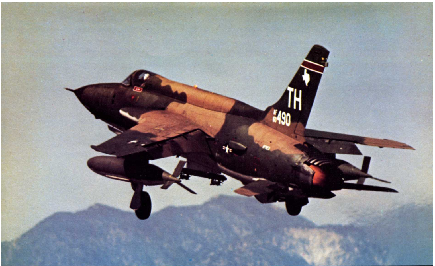
Above: Roaring out on take-off, its afterburners glowing, the F-105D, equipped with the Thunderstick II bombing system, first flew in 1969. T-Stick II included a special electronics system that was housed in a saddle-back fairing above the fuselage. (Compare with the older F-105B below.) Aircraft was operated by Texas ANG. (Peter Mancus/Cloud 9)
