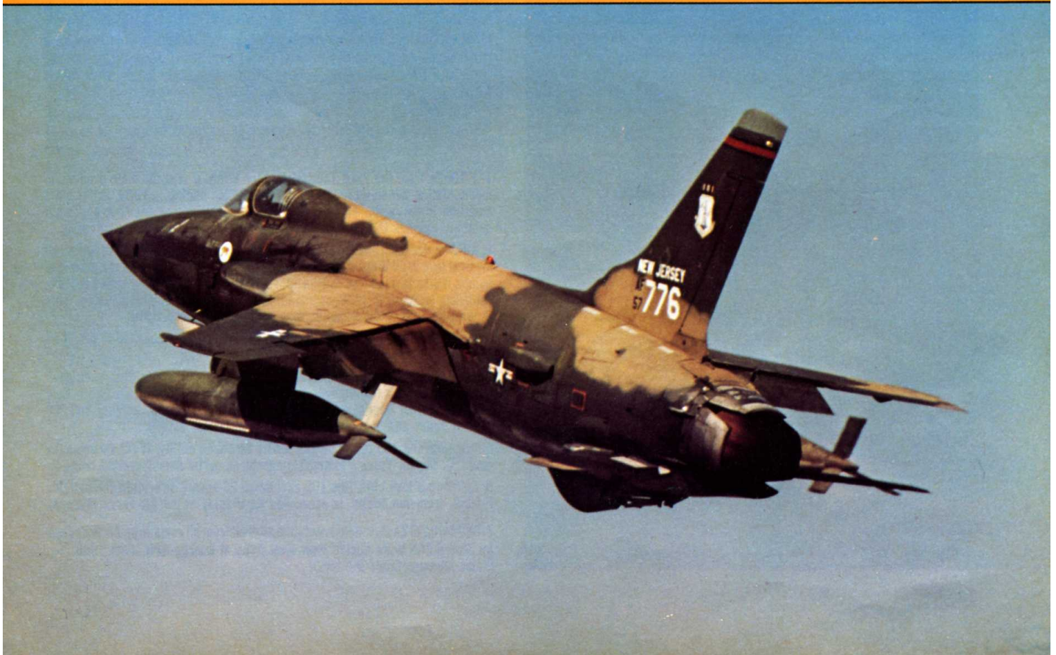
Below: A New Jersey ANG F-105B, one of 75 completed with larger J75-P-3 engine; the two original prototypes featured smaller J57 engines, without the elongated swept-forward air intakes. (Peter Mancus/Cloud 9)
