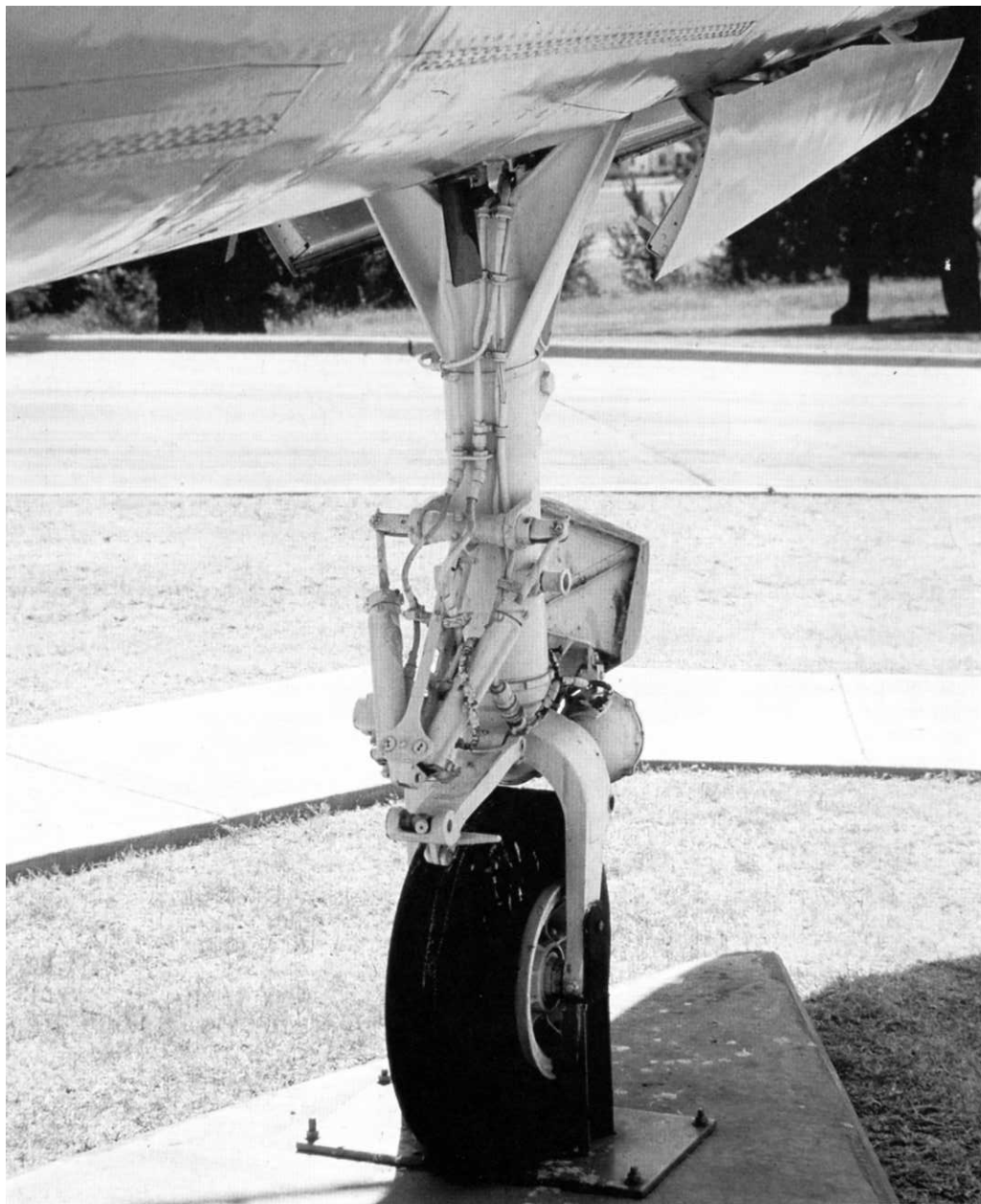
The F-105D and other Thunderchief variants used the same nose landing gear assembly. The gear strut retracted forward into its bay and was enclosed by two doors. A single wheel and tire was mounted on the strut. This restored F-105D's gear assembly is painted Gloss White (FS17875), which replaced the original Aluminum (FS17178) finish from the late 1960s. (Glen Phillips)
