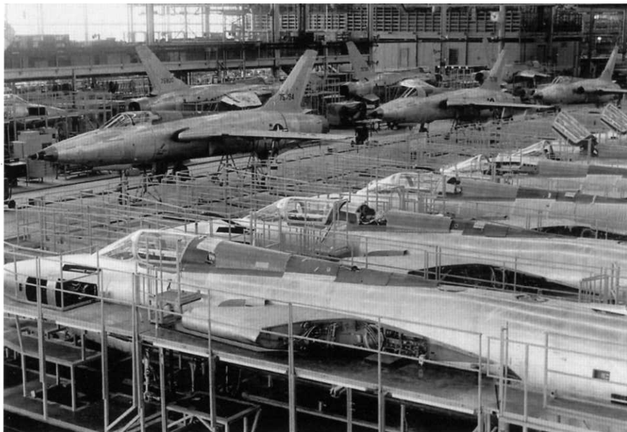
F-105Bs proceed through the final assembly area of Republic's Farmingdale plant in January of 1959. Fuselages lined up in the foreground await final component installation before they are mated to the wings and tail. Republic built 75 F-105Bs between 1956 and 1959, before switching to the improved F-105D. (Cradle of Aviation Museum)
