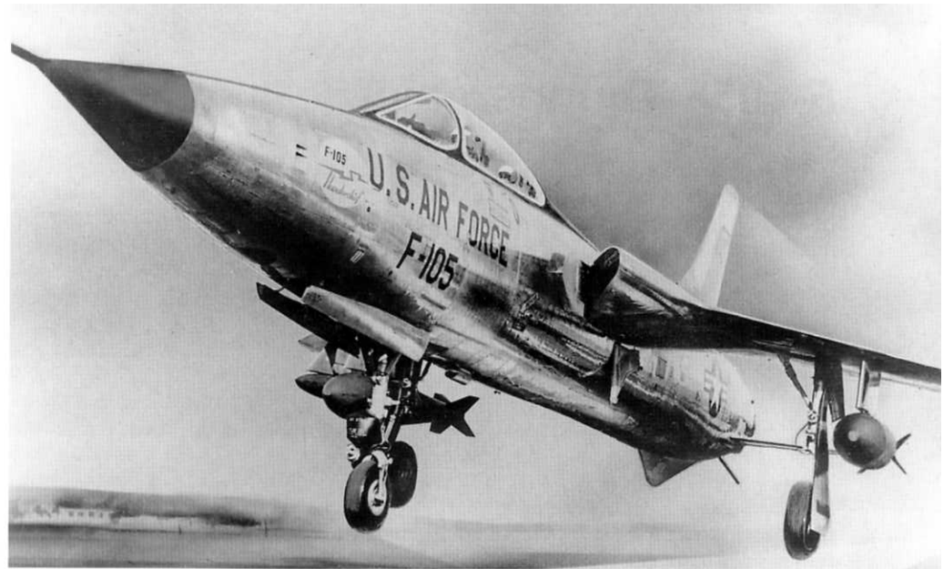
A Republic artist's conception shows the F-105E Thunderchief taking off, armed with bombs on the wing pylons. This two-seat trainer variant was proposed in 1958 and was the same length as the F-105D. A single Plexiglas canopy was designed to cover both crewmen. (Cradle of Aviation Museum)
