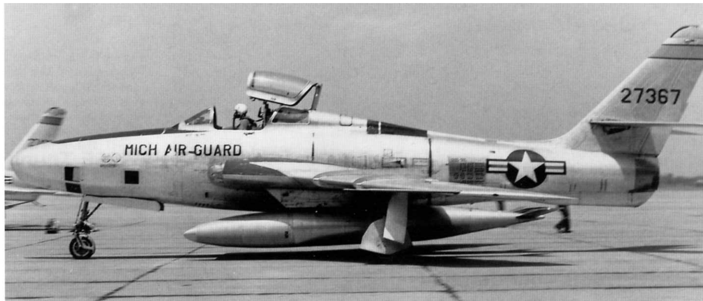
The RF-84F Thunderflash was based on the F-84F, but moved the engine inlet from the nose to the wing roots. This allowed photo reconnaissance equipment to be fitted in the nose. This taxiing RF-84F (52-7367) was assigned to one of two Michigan Air National Guard (ANG) Tactical Reconnaissance Squadrons between 1958 and 1971. (Cradle of Aviation Museum)
