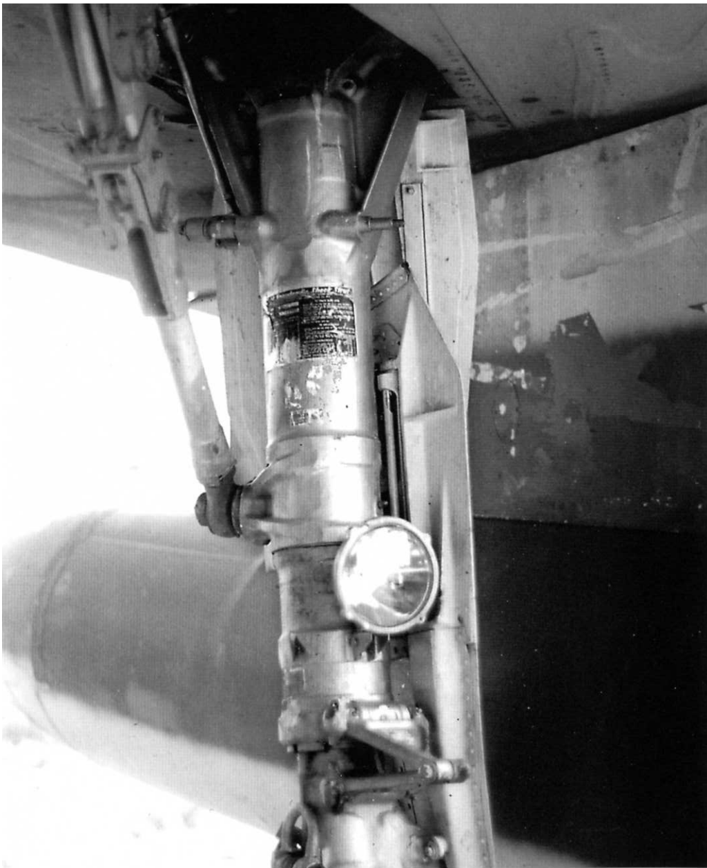
The F-105G main landing gear assembly was the same as the unit installed on earlier F-105D and F-105F variants. A strengthened structure was used to handle increased aircraft weights compared to the earlier F-105B. The main gear strut retracted inwards into the lower wing surface. A landing light was mounted on the strut's front, just above the scissor link connecting the upper and lower strut assemblies. (Ken Neubeck)
