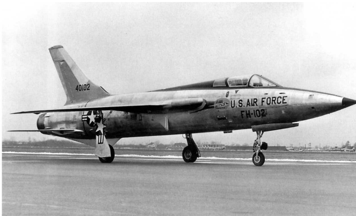
The third F-105B (54-0102) is parked on the runway of Republic airport in Farmingdale, Long Island in 1957. Thunderchief was first bestowed on this F-105 variant and appropriate artwork was painted on the aircraft's nose for its testing program. The small radome on the nose housed the E-34 ranging radar antenna. (Cradle of Aviation Museum)
