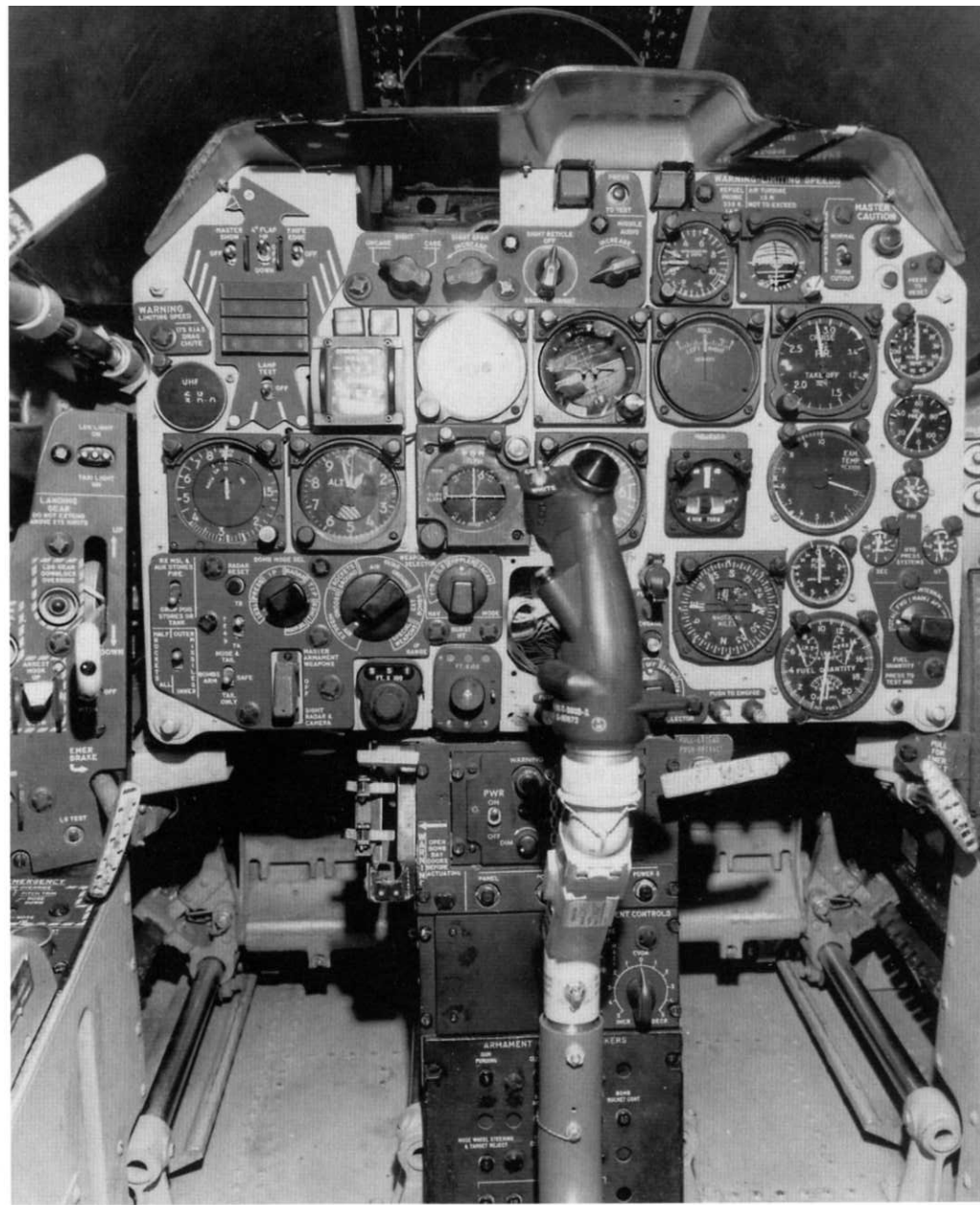
The F-105B cockpit consisted primarily of standard Air Force design. The rudder pedals traveled on metal bars located along the cockpit sides. This F-105B was one of nine assigned to the USAF Thunderbirds in 1964 and had modified flight control system instruments fitted to the upper port panel section. Thunderchief cockpits were primarily Cockpit Gray (FS36231) and Instrument Black (FS37038). (Cradle of Aviation Museum)
