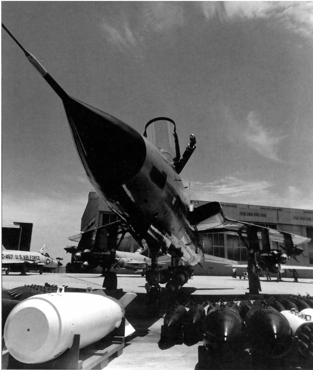
An F-105D is displayed with the variety of ordnance it could carry placed in front of the aircraft. AGM-12 Bullpup Air-to-Surface Missiles (ASMs) are mounted on the outboard wing pylons, while 500 pound (226.8 kg) bombs are loaded on the outboard wing and centerline racks. The Thunderchief's refueling probe is extended from its position on the port nose, ahead of the windshield. The light colored device ahead of the F-105D is a tactical nuclear 'shape' (inert weapon), which was usually carried in the weapons bay. (Cradle of Aviation Museum)
