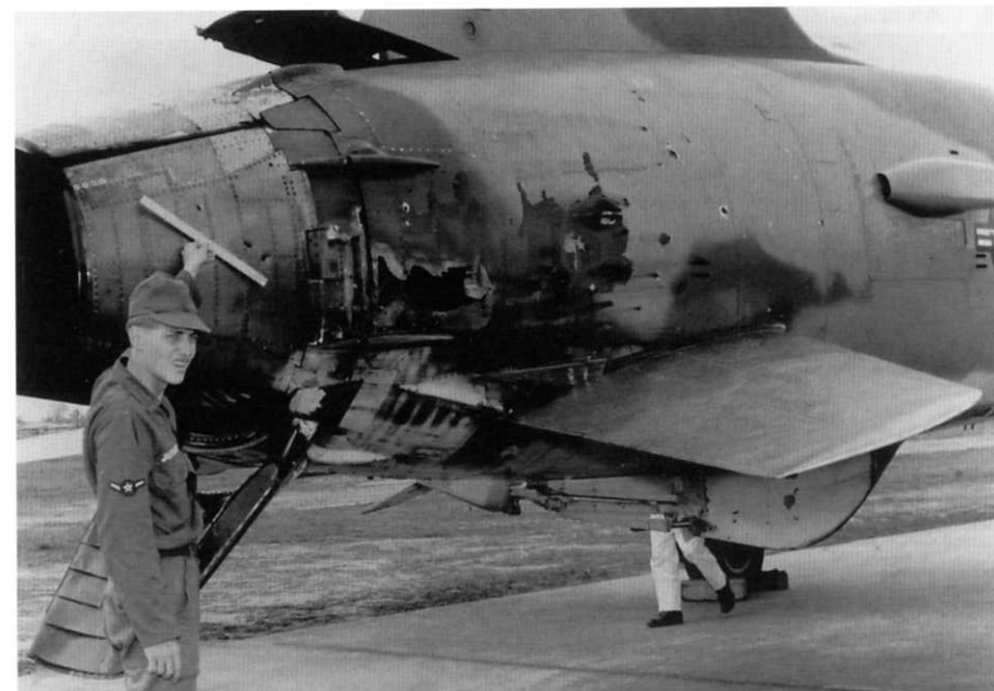
An airman places a ruler alongside the exhaust nozzle/speed brake of an F-105D (60-450) in July of 1967. This Thunderchief was hit by a North Vietnamese V-75 Dvina (SA-2 Guideline) Surface-to-Air Missile (SAM). The ruler provides scale for the shrapnel damage inflicted on the F-105D, which was able to safely return to its base. (Cradle of Aviation Museum)
