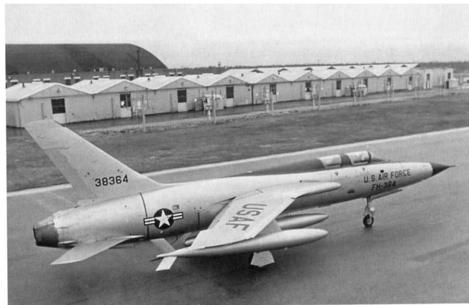
An F-105F (63-8364) prepares to take off from Republic Airfield on 9 January 1965. A 450 gallon (1703.4 L) fuel tank is mounted under the starboard wing and a 650 gallon (2460.5 L) tank is fitted to the centerline. F-105Fs were originally finished in aluminum lacquer (FS17178), with Olive Drab (FS34087) anti-glare panels on the upper fuselage. (Cradle of Aviation Museum)
