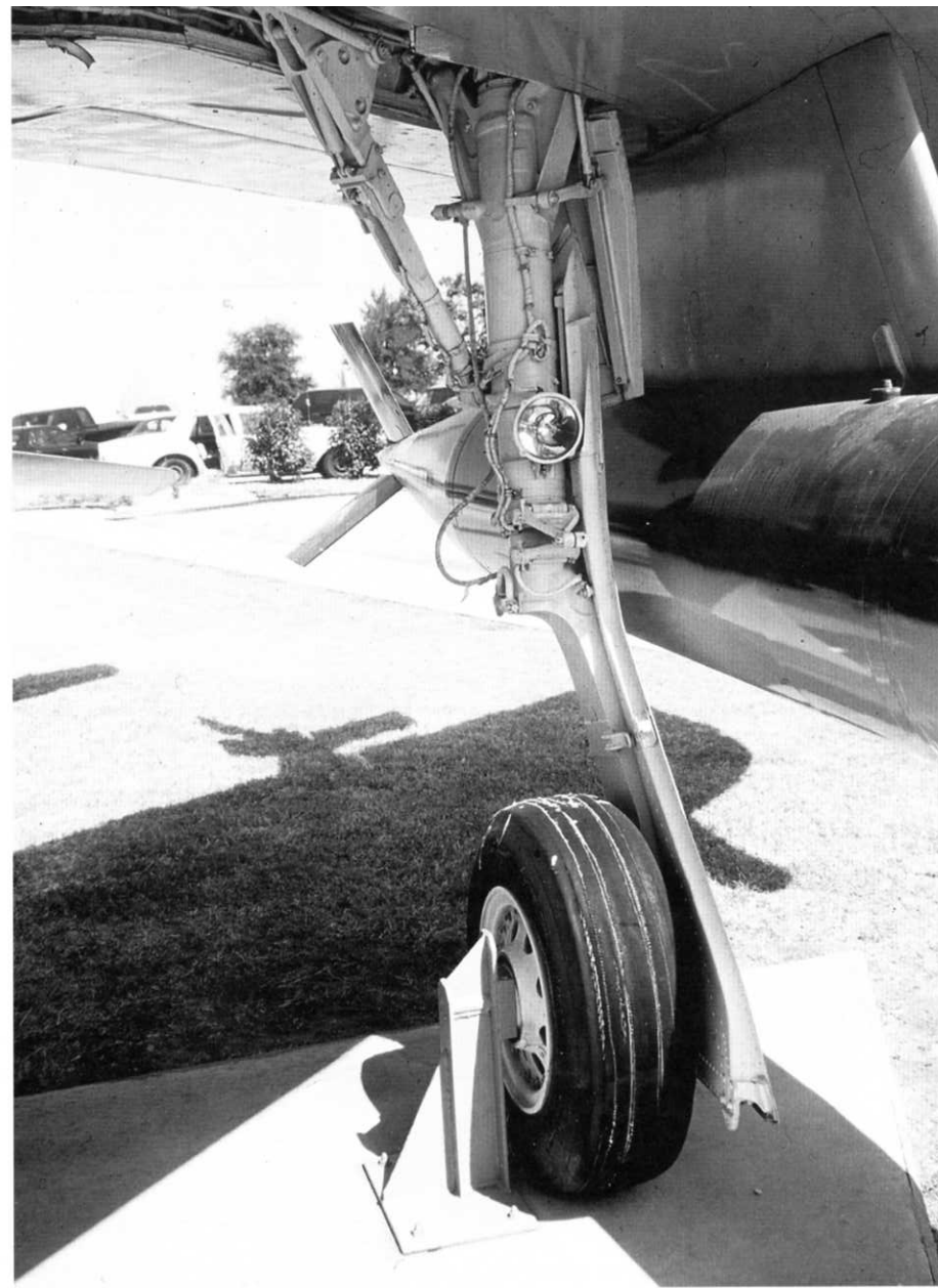
Thunderchief main landing gears were mounted in the inboard wing sections and hydraulically retracted outboard into their bays. A retraction strut from the bay connected to the main strut above and aft of the taxi light. The F-105D strut assembly appeared similar to the one fitted to early F-105Bs, but was strengthened to handle higher aircraft weights. The wheel and tire on this restored example are raised off the ground to reduce wear on these items. (Glen Phillips)
