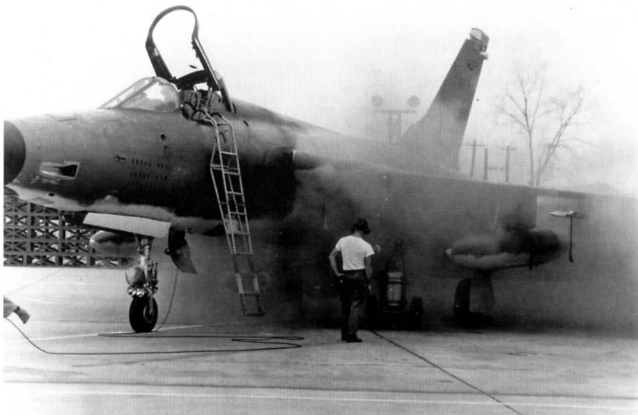
Ground crew at Korat RTAB, Thailand install a new J75-P-19W engine into the F-105D's fuselage. The powerplant was wheeled into position on a Model 4000A trailer, which employed hydraulic control for raising and lowering the engine. The Thunderchief's fuselage split in two aft of the wing trailing edge, with the engine fitting inside the aft section. J75s were normally changed at every 200 flight hours; however, constant high speed and low altitude flying in Southeast Asia reduced this time to 125 hours. (Cradle of Aviation Museum)
