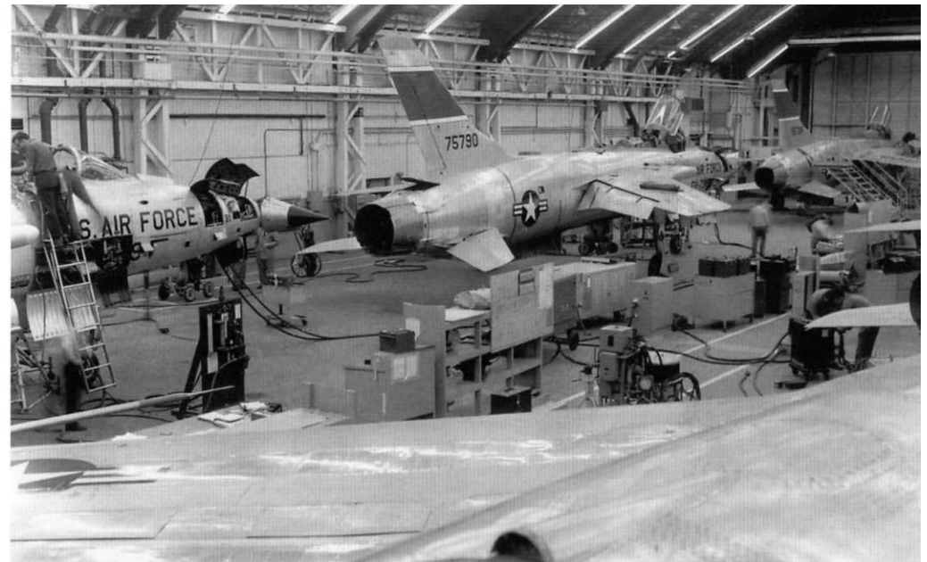
Technicians check completed F-105Bs in the final assembly area at Farmingdale. The brake parachute compartment door is open near the tail of 57-5790. These Thunderchiefs would perform company flight tests before Republic delivered them to the US Air Force. The nose and tail bands are believed to be green (approximately FS14110) and white, indicating their assignment to the 335th TFS, 4th TFW. (Cradle of Aviation Museum)
