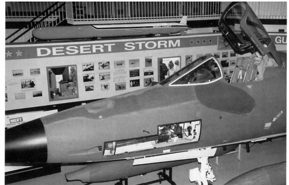
The F-105D's nose was increased 16.3 inches (41.4 cm) from the earlier F-105B's nose. This extra space was filled with additional avionics equipment, which gave the F-105D an all-weather capability. The 20mm cannon was retained in the same location as on the F-105B, but the lengthened nose placed the muzzle further aft of the radome. This restored Thunderchief is displayed at the Eglin AFB Museum in Valparaiso, Florida. (Dennis R. Jenkins)
