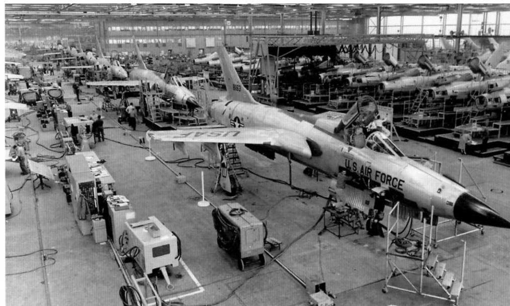
An F-105D-5-RE (58-1163) leads a row of Thunderchiefs on the final assembly line at Republic's Farmingdale plant in early 1960. Technicians install electrical and hydraulic components into the lower starboard fuselage. Fuselages of other F-105Ds await component installation before wings and tail surfaces are mated to them. (Cradle of Aviation Museum)
