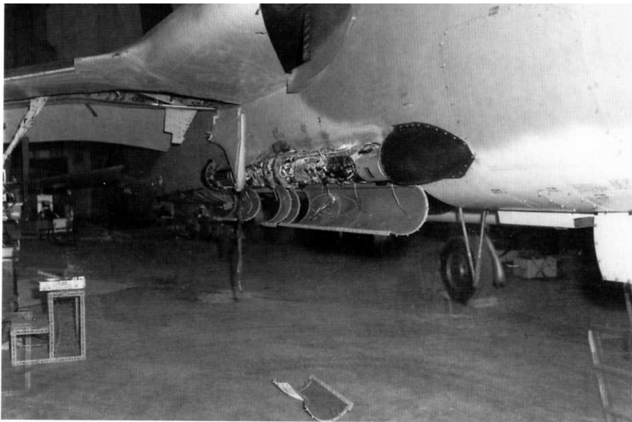
Covers for the starboard AN/ALQ-105 ECM pod were opened on this F-105G undergoing maintenance. These covers allowed technicians to access the pod's electronic assemblies and wiring for servicing. Westinghouse split one of its AN/ALQ-101 pods in half to create the AN/ALQ-105 for the F-105G. This installation freed a wing pylon for ordnance. (Cradle of Aviation Museum)
