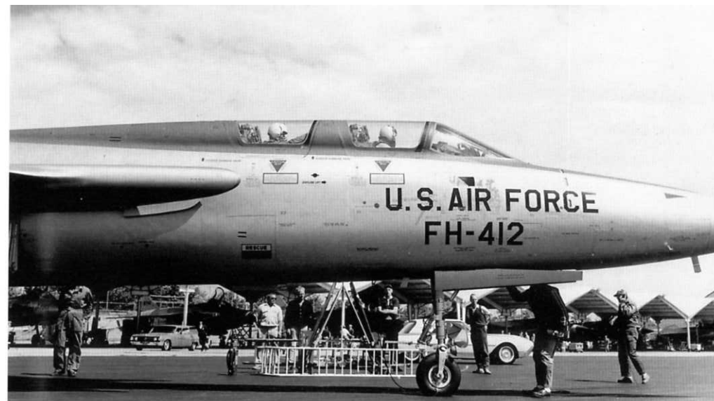
Air Force flight and ground crews prepare the initial F-105F (62-4412) for its delivery flight from Farmingdale on 21 June 1963. One of the crewmen inspects the nose landing gear bay for any problems. The F-105F's fuselage was lengthened 30.7 inches (78 cm) to accommodate the second seat, while retaining the F-105D's internal fuel capacity of 1026 gallons (3883.8 L). (Cradle of Aviation Museum)
