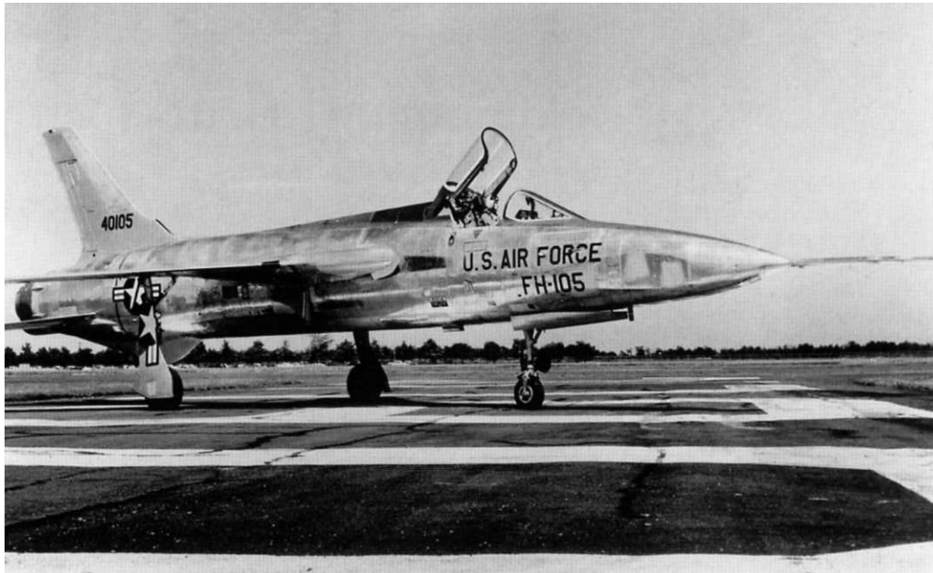
The first of three JF-105B test aircraft (54-0105) taxis toward the active runway in 1957. The JF-105Bs were originally ordered as RF-105A reconnaissance aircraft, but this program was cancelled in 1956. These Thunderchiefs had the photo windows covered over and test equipment fitted inside the nose. (Cradle of Aviation Museum)
