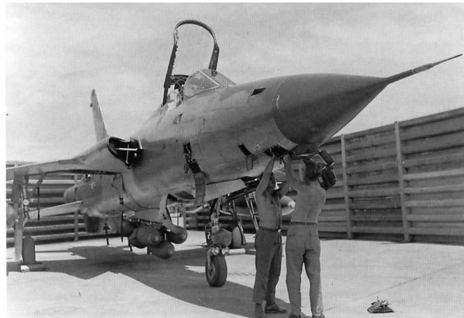
USAF maintenance personnel change strike camera film in the nose of an F-105D at Korat RTAB. The rear-facing motion picture camera recorded attack run results for later study. Thunderchiefs were housed in open-air revetments at their Thai bases to reduce the risk of attack by Communist irregular forces. Six 750 pound bombs are loaded on the MER fitted to the centerline pylon. (Cradle of Aviation Museum)
