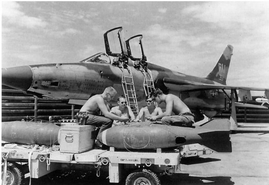
Ground crew prepare to load 750 pound M117 bombs onto a 354th TFS F-105F (RM/63-8351) at Korat RTAB. The Olive Drab (FS34087) bombs have Orange Yellow (FS33538) nose rings to indicate high explosive weapons. Thunderchiefs carried up to six M117s on a MER mounted on the centerline pylon. A Shrike ARM is fitted to the port outboard pylon. (Cradle of Aviation Museum)
