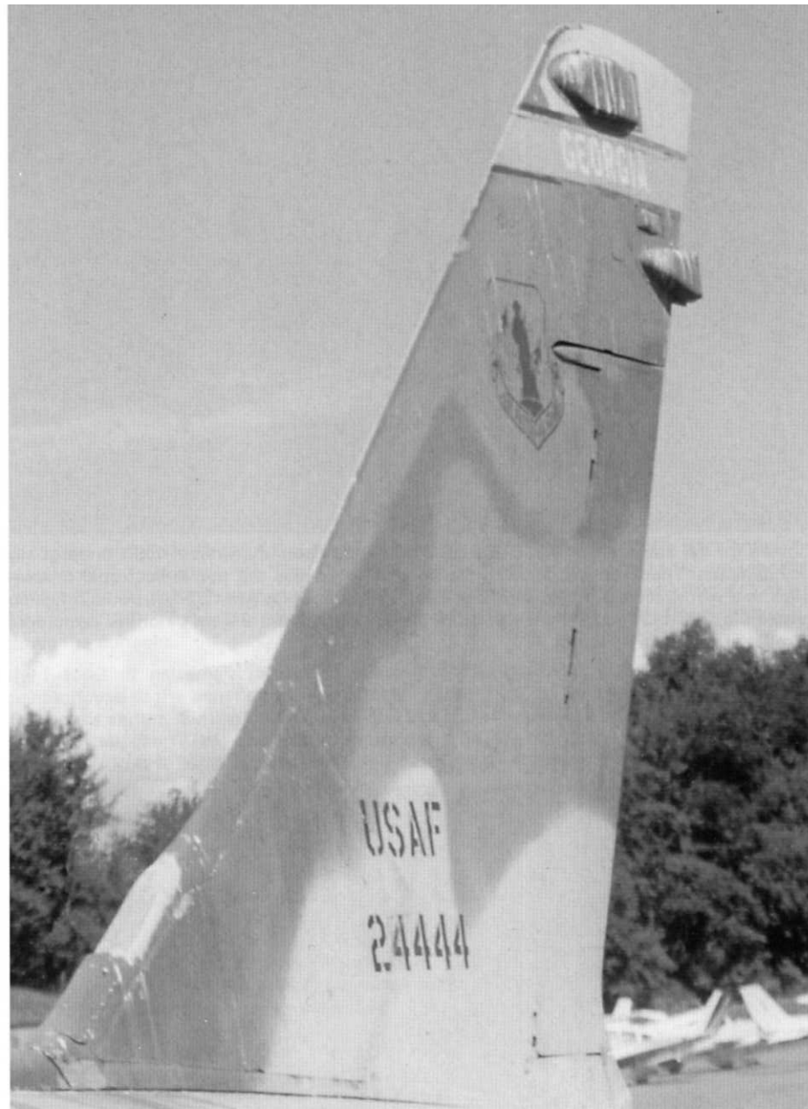
F-105Fs and Gs had their vertical tail sections increased by five inches (12.7 cm) and their base chord (width) widened. These measures provided additional stability for a longer aircraft than previous variants. A cover was placed over the afterburner cooling air intake on the vertical stabilizer's lower leading edge. Antennas for the AN/APR-25/26 RHAW system were retrofitted on the vertical tail. This F-105G (62-4444) served with the Georgia ANG until retirement in 1983. (Cradle of Aviation Museum)
