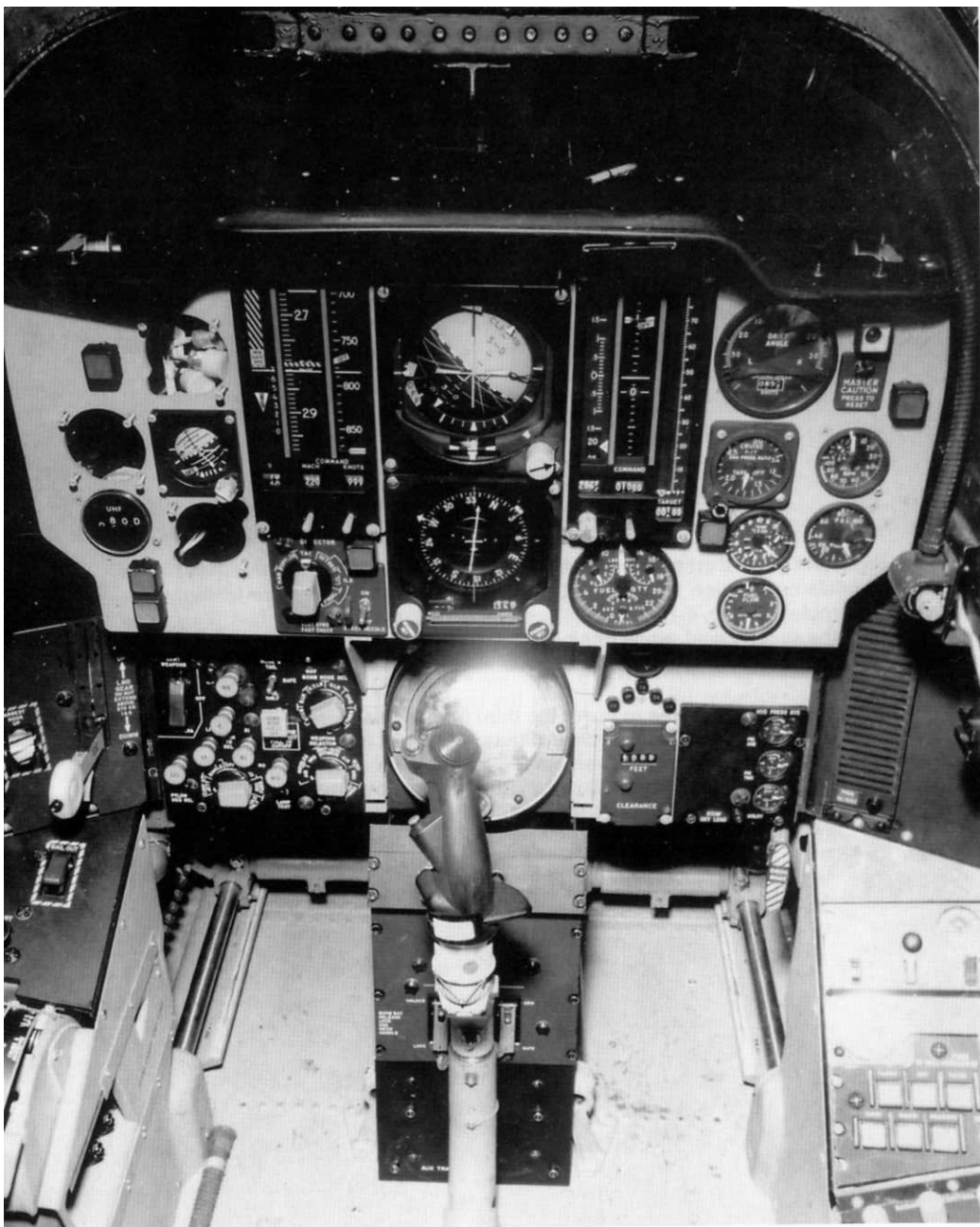
The F-105F's aft cockpit had fewer instruments than the forward cockpit, which was identical to the F-105D cockpit. The light blue and black artificial horizon was mounted on the upper center of the panel. Full flight controls were provided to allow the occupant – either an instructor pilot or an Electronic Warfare Officer (EWO) on Wild Weasel missions – to fly the F-105F if the pilot was incapacitated. (Cradle of Aviation Museum)
