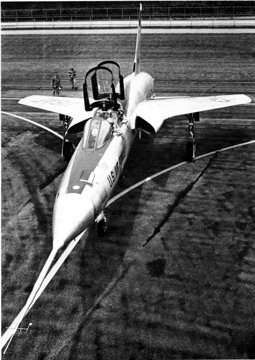
Initial example of the F-105F series, outfitted with test boom on nose. (Republic)
