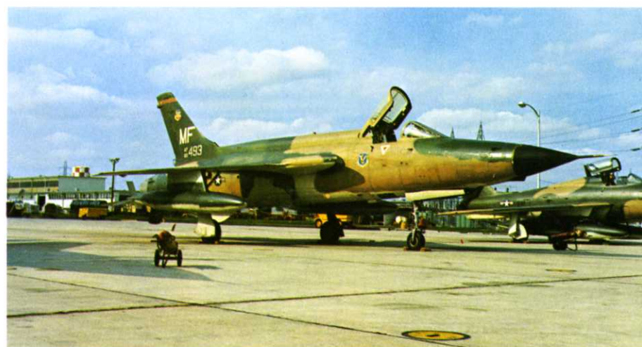
F-105D-10-RE of the 563rd TFS, 23rd TFW. One of the D's retrofitted with the 'Thunderstick II' avionics saddleback. (Norman E. Taylor)
