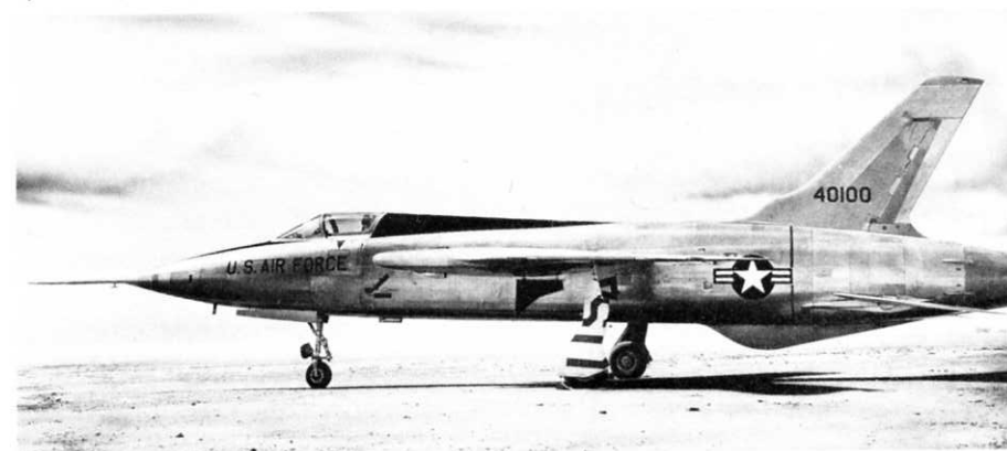
The second YF-105A on the ground at Edwards AFB in May 1956. (above) First two F-105B's (left and below) The "B" models incorporated many advancements in existing "state-of-the-art" aircraft design, including the area ruled fuselage, and the J-75-P-3 Engine. Also introduced with the "B" were the swept-forward intakes, which help in directing a constant flow of air to the engine over a wide range of speeds. (USAF)
