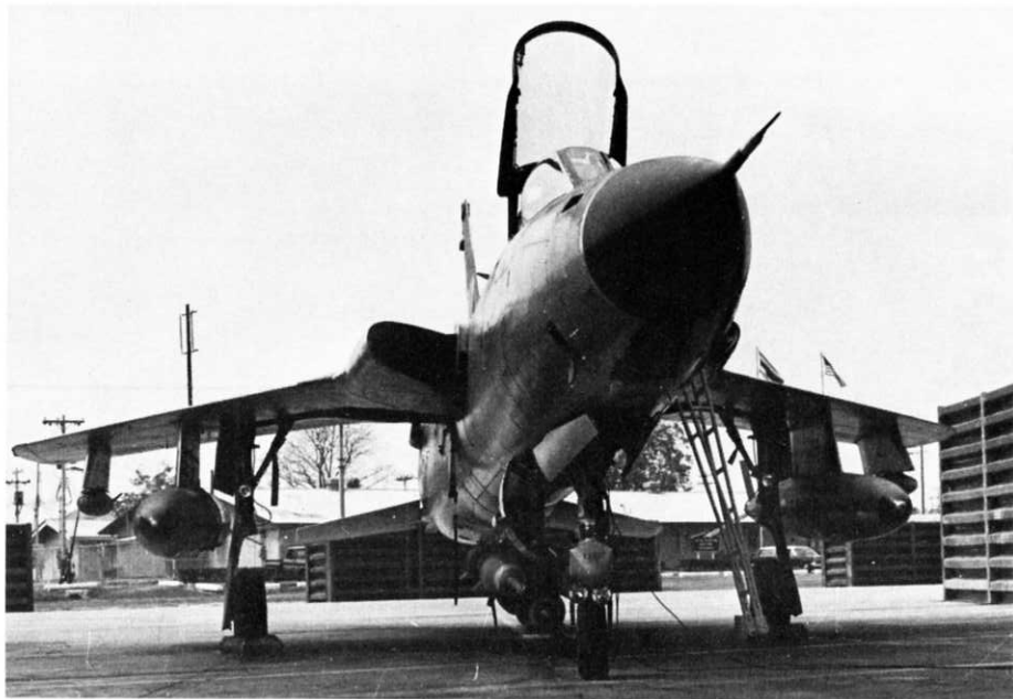
Thud of the 355th TFW in revetment at Takhli February, 1970. It is loaded with 750 lb. bombs on centerline, and 500 lb. bombs outboard. (USAF)
