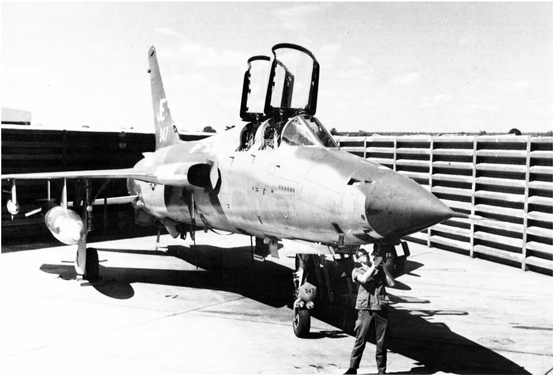
44th TFS Wild Weasel gets a fresh film cartridge for it's strike camera at Korat RTAB, 1969. Other access doors open on the left side of the nose are for Hydraulics systems accumulators, and utility hydraulics reservoir filler. Performance figures of the "F" model Thud are within 3% of those for the "D", main difference being in dimensions. (The "F" is 5'3" longer, and 6" taller.) (USAF)
