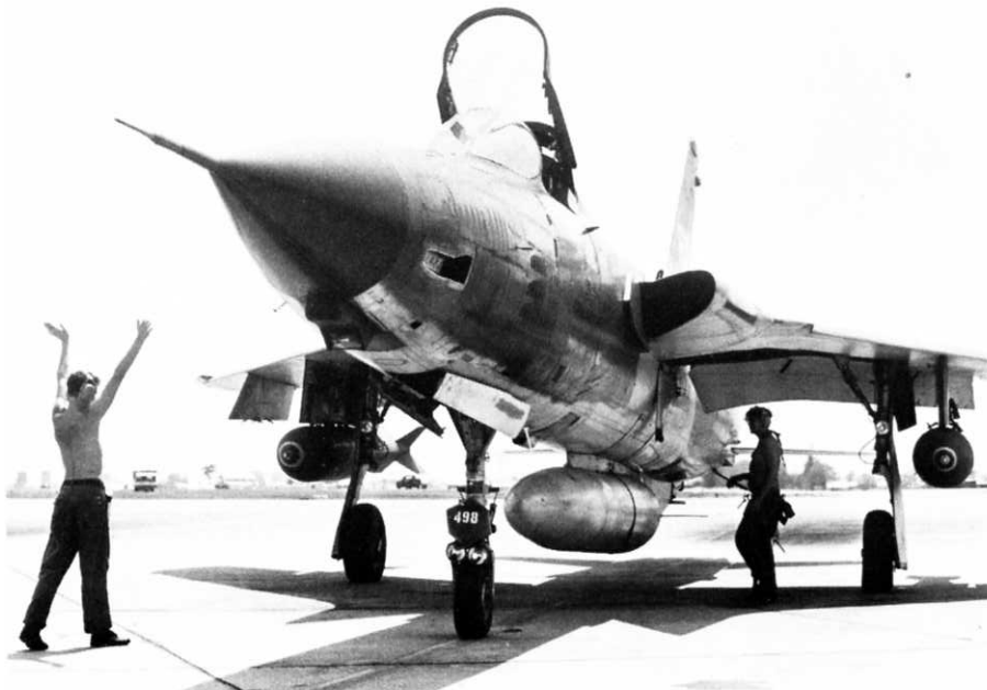
Thuds with diverse ordnance loads. 498 carries 3,000 lb. bombs, used against "hard" targets, while 344 carries cluster bomb units and Mk 81's for use against personnel. Both assigned to 355th TFW at Takhli in 1970. (D.M. Weaver via Jim Farmer)
