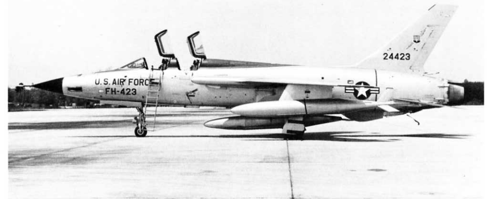
F-105F-1RE . Note that vertical fin of the "F" is taller than that of other Thunderchief variants. (Norman E. Taylor)
