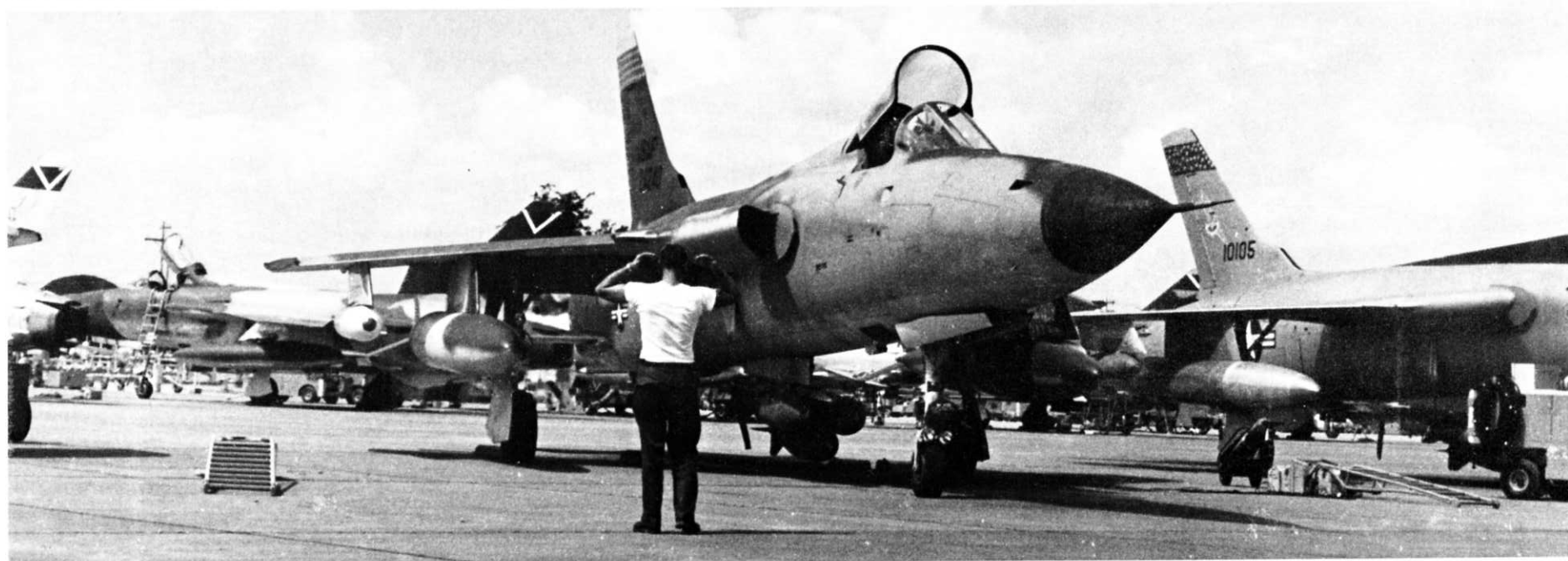
4th TFW F-105D's beginning a mission against North Vietnam in 1965. Early in the air war against North Vietnam, Thuds carried rockets on outboard pylons. Radar directed AAA and SAM's forced Thuds to start carrying ECM gear later in the war. (USAF)
