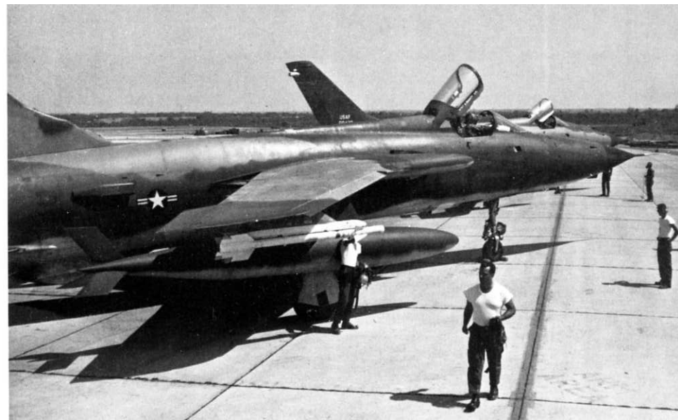
Thud of the 44th TFS in the arming area prior to mission over North Vietnam. As the Mig threat became more serious, 105's started to carry a Sidewinder on one pylon, and an ECM pod on the other. (Dan Cherry)
