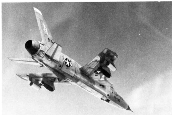
F-105D-5-RE , carrying 750lb. bombs and rocket pods. Note that the arresting hook has not been installed, and it still sports the natural metal finish typical of pre "Operation Look-Alike" Thunderchiefs. (Republic)
