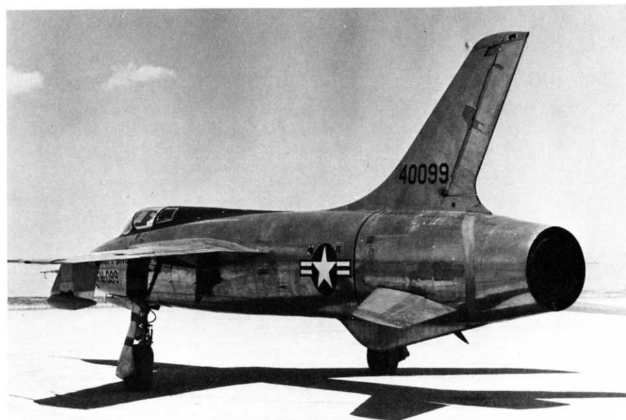
The first Thunderchief , the YF-105A, taxis out for a test flight at Edwards AFB, 31 October, 1955. Note the "straight" air intakes. (USAF)
