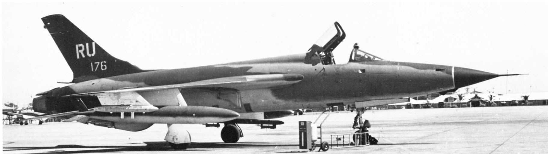
F-105D , of the 357th TFS, 355th TFW, out of Takhli RTAB was photographed at Ubon RTAB in March 1968. ECM pod on outboard pylon, MER on centerline. (Al Piccirillo via Norman E. Taylor)
