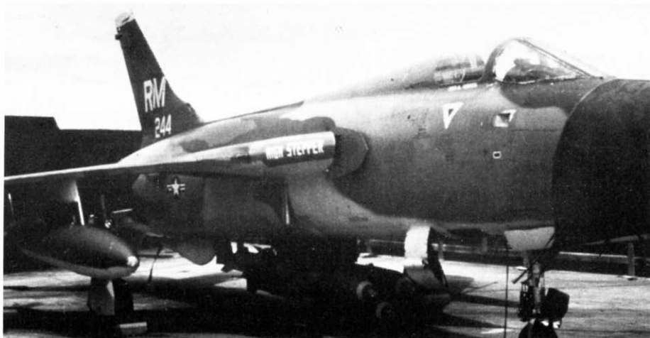
"High Stepper" was F-105D, 62-4244, of the 355th TFW at Takhli RTAB, August, 1970. Canopy Frames and background for name were medium blue. Open access door behind nose gear is for Auxiliary Electronics Compartment. (Don Jay via Lars Soldeus)
