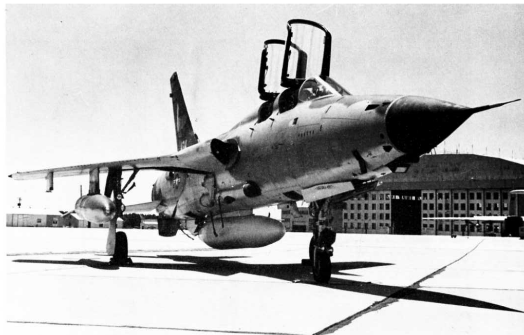
F-105F at Eglin AFB during testing of the QRC-380 ECM blisters on fuselage sides, 1970. (USAF)
